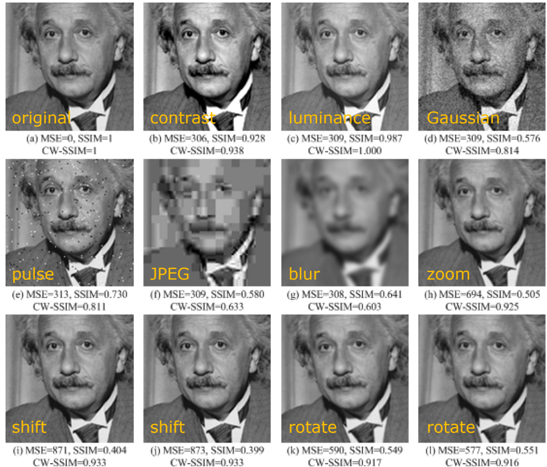
[FIG2] Comparison of image fidelity measures for "Einstein" image altered with different types of distortions. (a) Reference image. (b) Mean contrast stretch. (c) Luminance shift. (d) Gaussian noise contamination. (e) Impulsive noise contamination. (f) JPEG compression. (g) Blurring. (h) Spatial scaling (zooming out). (i) Spatial shift (to the right). (j) Spatial shift (to the left). (k) Rotation (counter-clockwise). (l) Rotation (clockwise).
